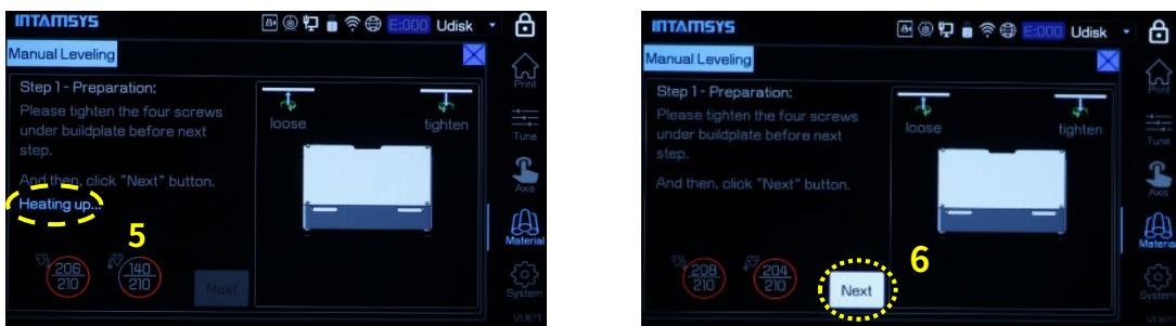
**STEP 4:** There are 4 screws which need to be adjusted one by one for at least twice, by using the leveling card with 0.2mm thickness (the leveling card is in the accessory box).
