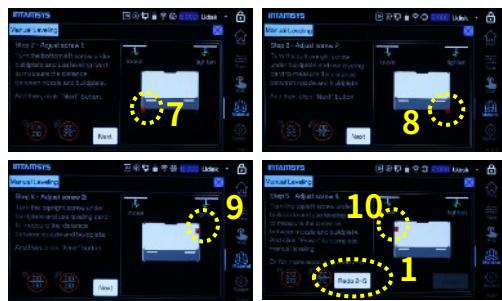
**STEP 5:** Press “Finish” to exit the process after adjustment is completed.
