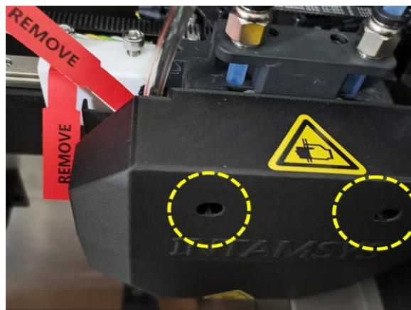
**STEP 6:** Cut the tie around the nozzle and remove it, then install the front cover back to the original place.
